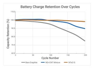
NTeC in batteries demonstrates longer life than traditional or simple mixture chemistries
