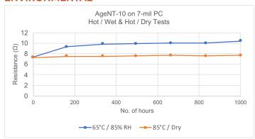
Resistance, adhesion and optical properties exhibit very stable behavior with environmental aging.
