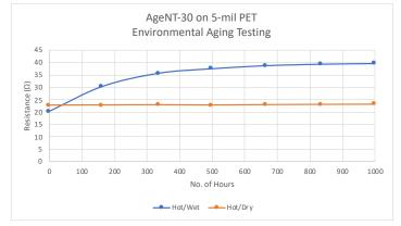
Resistance, adhesion and optical properties exhibit very stable behavior with environmental aging.
